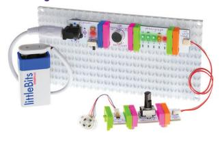
The mounting board allows students to keep their circuit intact and move it around with ease. Students snap together their littleBits circuit and press the feet of the Bits into the holes of the mounting board. Mounting boards also provide an effective way for students to store their circuits safely between work sessions.
