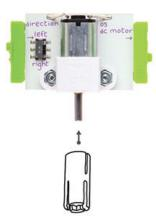
The MotorMate is an accessory included with the DC motor that makes it simple and easy to attach wheels, paper, cardboard, gears, and other materials to the 'D' shape of the motor shaft.
